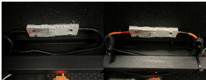
3. Strip both wire leads (hot, neutral and ground) just enough to attach to your inverter as needed without any exposure once connected. Ensure connections are tight and secure.
