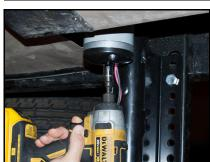
To override the stabilizer jacks. Locate the <sup>3</sup>/<sub>4</sub>" nut on the out facing end of the stabilizer jack. Use a 3/4 "socket or wrench to raise or lower the jacks.
