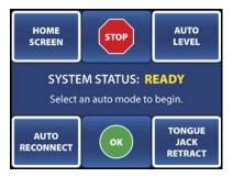
Press **OK** to begin "TONGUE JACK RETRACT" or **STOP** to make another selection. The display will read "TONGUE JACK RETRACT IN PROGRESS". When the jack has been fully retracted the display will read "TONGUE JACK RETRACT SUCCESSFUL" and a beep will sound.
