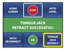
Raise all adjustable feet to the hole that provides the most ground clearance before towing the unit. Press **ON/OFF** to deactivate the display. **WARNING:** Visually check all jacks to ensure that they are fully retracted before towing the unit. Close and latch the cover of the touch screen display.
