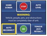
The system will retract all stabilizer jacks and the rear leveling jacks, then extend or retract the tongue jack until the proper connection height is achieved. The display will read "AUTO RECONNECT IN PROGRESS". When the system has completed the "AUTO RECONNECT" function the display will read "AUTO RECONNECT SUCCESSFUL" and a beep will sound.
