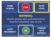
The system will go through a series of moving the jacks and checking the unit for level. The display will read "AUTO LEVEL IN PROGRESS". When the system has successfully leveled the unit, the display will read "AUTO LEVEL SUCCESSFUL" and a beep will sound.
