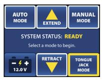
Press **AUTO LEVEL**. **WARNING**: Vehicle, people, pets and obstructions must be completely clear of unit before executing the "AUTO LEVEL" function. Press **OK** to begin "AUTO LEVEL" or **STOP** to make another selection.
