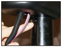
Rear Leveling Jacks – With the jack extended half way remove the plastic plug and apply
