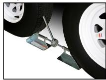
Press **ON/OFF** to activate display. Press **TONGUE JACK MODE**. Press and hold **EXTEND** until the necessary detachment height is reached. Disconnect, and pull the tow vehicle completely clear of the unit. Lower the rear leveling jack adjustable feet and position them so that they are close to the same distance from the ground. Press **AUTO MODE**.
