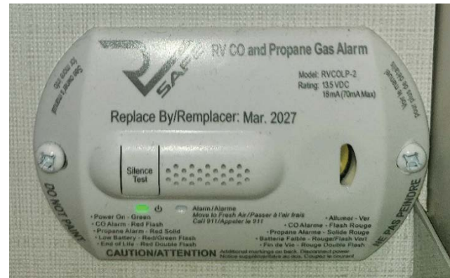
THE CO AND PROPANE GAS ALARM. SEE SECTION 4H FOR ITS LOCATION IN THE RV.
