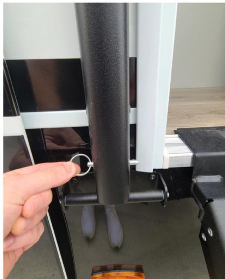
2. There is an inner and outer channel that comprises the handrail. Once the handrail is extended in step (1), firmly grab the inner channel located at the bottom of the handrail and pull it down and outward until the inner channel is fully extended.
