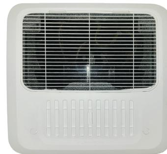
Over time, the A/C gasket will need to be replaced. To gain access to the mounting bolts, the A/C shroud and filter from inside the RV will need to be removed. From there you will be able to carefully remove the bolts and gain access to the seal itself.
