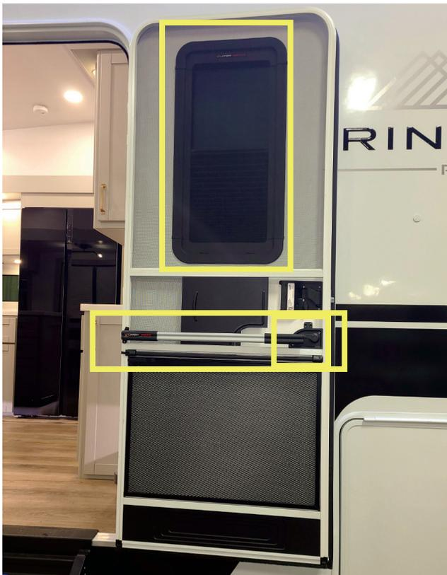
**2. Lippert Screen Shot**—The middle yellow rectangle highlights two features of the entry door. The first is the Lippert Screen Shot. This is the black tube that runs parallel to the ground below the door latch. It has a spring-loaded strap that automatically shuts the screen door after it has been opened.
