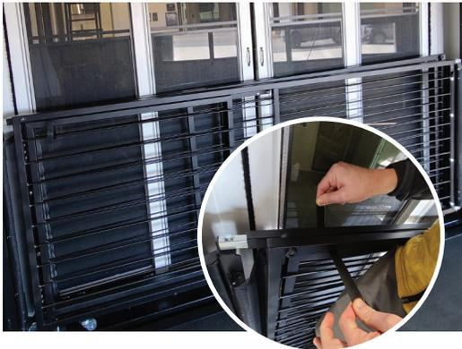
5. Starting with the first outermost section of the patio rail kit, carefully swing the rail towards the edge of the ramp door.
