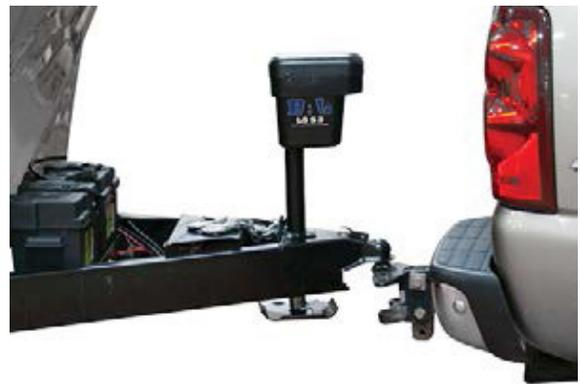
5. Raise all adjustable feet to the hole that provides the most ground clearance before towing the unit. Press **ON/OFF** to deactivate the display.
