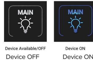
Buttons for Slides and Awnings are “momentary.” They activate the device only when the button is being pressed. When the button is released, the device returns to the “Off” position automatically. This provides safety by requiring the switch remain held by an operator during activation.
