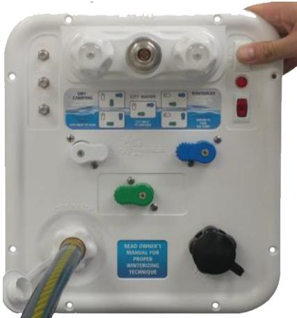
20. **CONNECT** a short section of garden hose to the inlet labeled “**CITY WATER**” on the convenience center panel and as shown in the picture immediately above.
