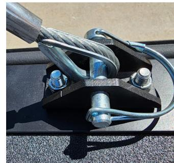
3. After locating these plates, remove the D-ring pin holding the cable in place.
