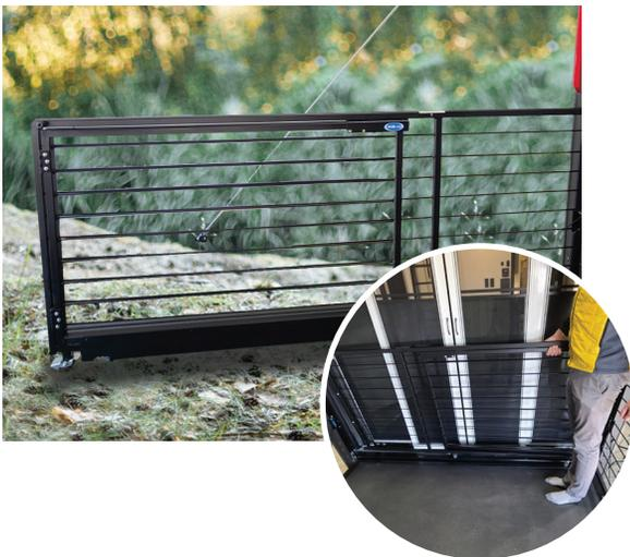
10. Pivot the door side rail towards the RV until it meets the other rail. Once the off door (driver) side rail is close to the other, you will need to slightly lift the rail to set it into its proper closed position.
