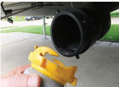
2. Open black waste holding tank and leave open to allow black tank to drain.
