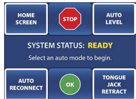
4. Press **OK** to begin “**TONGUE JACK RETRACT**” or **STOP** to make another selection. The display will read “**TONGUE JACK RETRACT IN PROGRESS**”. When the jack has been fully retracted the display will read “**TONGUE JACK RETRACT SUCCESSFUL**” and a beep will sound.
