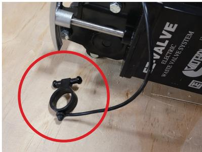
To reengage electric valves, push handle all the way in to close the valve, rotate the Valterra handle 90 degrees in opposite direction to original position, then replace black plastic ring on the valve.
