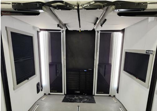
2. Close the inner 3-Seasons panels by sliding the inner panels together in the center of the opening.
