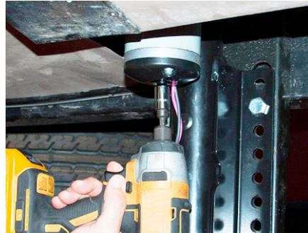
5. To override the stabilizer jacks. Locate the 3/4" nut on the out facing end of the stabilizer jack. Use a 3/4" socket or wrench to raise or lower the jacks.
