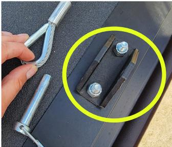
6. Place the cable eyelet between the plate verticals and insert the provided D-ring in the correct orientation and ensure it is secured with the supplied cotter pin. Please see below.
