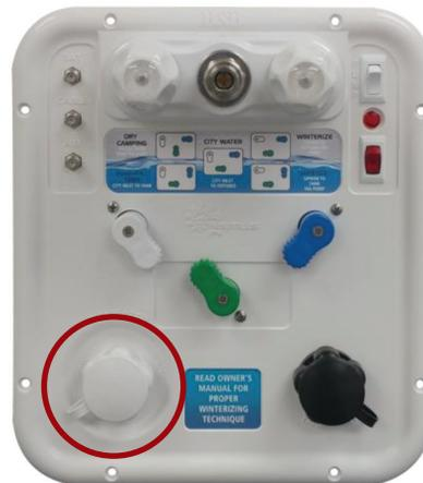
14. Using the **CITY WATER INLET** (located at the red circle shown in the picture above) on the convenience center panel:
