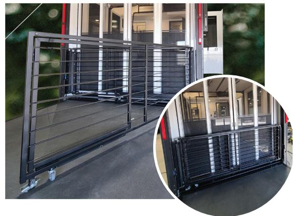
11. Prior to closing the ramp door, use the velcro strap to secure the two rails together.
