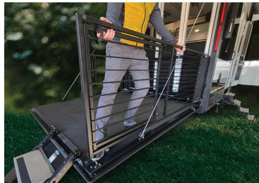
7. Once the rail is fully extended, engage the latching mechanism at the end of the railing as shown in the picture below.
