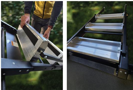
b. Press the two push releases in, and lift the stair up.
