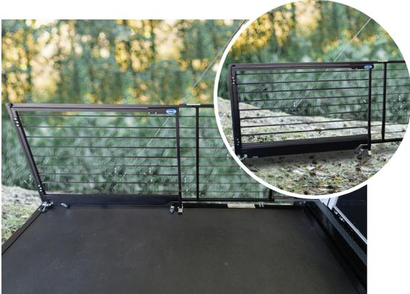
9. The off door side rail also contains the rail kit portion for the front or top of the ramp door. Pivot the front rail into place and engage the latch as indicated in the below photo.
