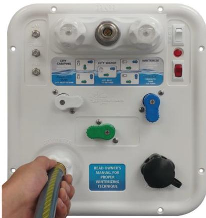
5. **TURN ON** the water pump and fill the fresh tank with the full amount of sanitizing solution. You can turn the water pump on at the convenience center (picture below left) or the control panel (picture below right):
