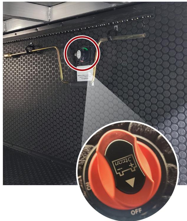
**The master, or main, battery disconnect** will prevent all draw coming from any component within the RV including those that are memory-based, or safety related. It kills power to everything. The master battery disconnect is in the front bulkhead (or firewall) storage area.
