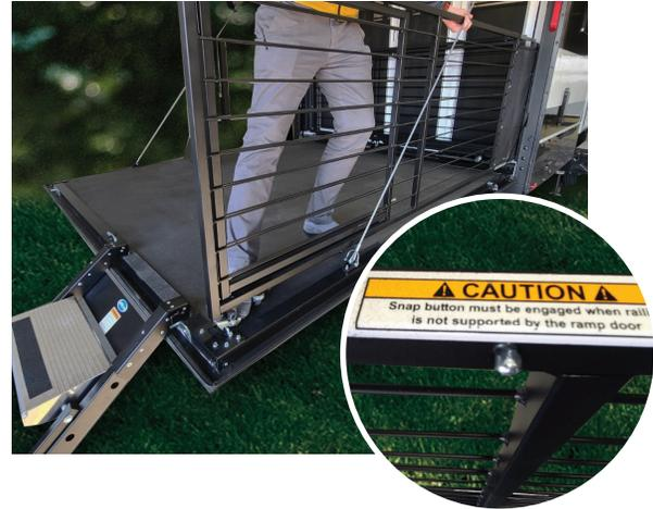
8. Pivot the off door (driver) side rail towards the RV. You will need to gently lift the rail while moving it towards the RV until it lays flush with the 3-Seasons door.
