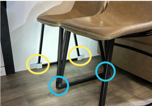
To secure dinette chairs for transit slide chair frame closest to slide out wall into attached metal chair brackets (circled in yellow). Use included velcro straps (2, circled in blue) to secure second chair to chair that has been secured in metal frame.
