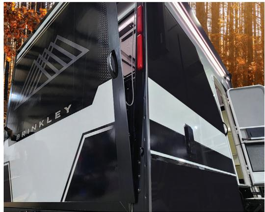
2. With one hand on the ramp door, insert the key and rotate counter-clockwise to release, or unlock, the ramp door.
