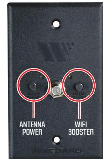
There is also an on and off button located to the right of the coax connection. This button is to turn the WiFi on and off. This button is utilized if the WiFi router is added in the aftermarket.
