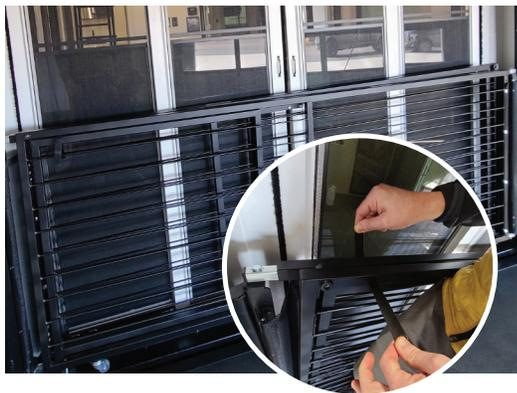
5. Starting with the first outermost section of the patio rail kit, carefully swing the rail towards the edge of the ramp door.
