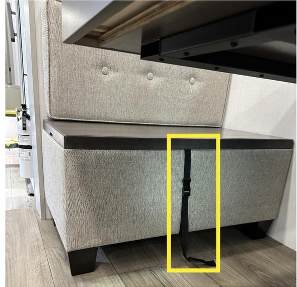
To secure ottoman for transit use black nylon securement strap with buckle (highlighted in yellow box) which is attached to the slide out wall. To secure ottoman wrap one side of the strap over the top of ottoman, while wrapping the other side of the strap underneath the ottoman, then secure plastic buckle. Strap may need to be adjusted to make sure it fits securely. To remove strap squeeze both tabs of buckle simultaneously and pull apart.
