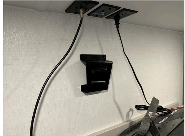
To reinstall TV line up sideways “V” shaped bracket on back of TV to the corresponding grooves on bracket attached to wall. Slide TV to the left until you hear TV bracket latch click and reengage. At this point the TV is now secured to wall bracket.
