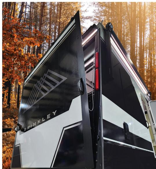
3. Guide the ramp door down to the desired position. If the support cables are connected to the ramp door, the door will only open to the patio mode position. To allow the door to fully rotate down to the ground, you must first disconnect the support cables from the ramp door on each side. Both positions are shown below.
