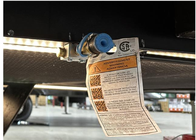
Your unit may be equipped with a quick connect LP port on the exterior of the unit. It is to be used for LP appliances such as grills etc. Please use caution when using any such appliance while it is connected to LP
