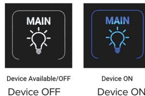
Buttons for Slides and Awnings are “momentary.” They activate the device only when the button is being pressed. When the button is released, the device returns to the “Off” position automatically. This provides safety by requiring the switch remain held by an operator during activation.
