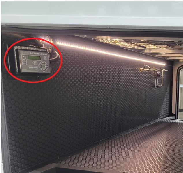
The Auto Leveling Touch Pad is located on top of the front jack on Travel Trailers.
