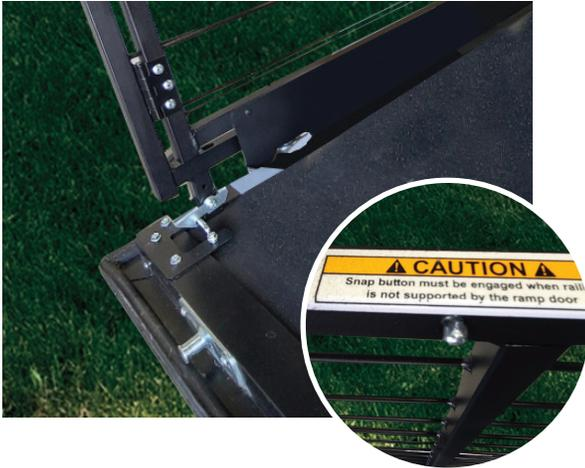
9. Locate the next foot latch on the door (passenger) side rail and press the latch down to release while pulling the rail straight back towards the RV until you hear the detention pin engage.
