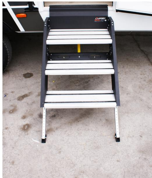
4. Adjust the extension legs of the step on both sides by pulling the provided pins and adjusting the leg lengths so that the step treads are parallel to the ground.
