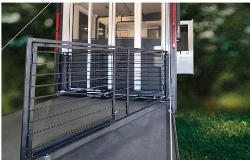
6. As the rail meets the edge of the ramp door, you will need extend the telescoping portion of the rail kit to the outermost corner of the ramp door. This is performed by grabbing the rail and guiding it towards the direction of the stairs.
