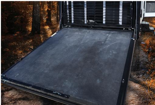
4. To close the ramp door, ensure the garage entry door is open. This will allow air to escape the garage as the ramp door closes.
