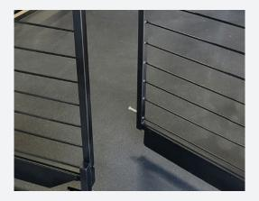
6. From there, start with the rail just left of the stairs (if you are facing the RV). Press downward on the foot latch to release the rail from the floor securement and pivot the rail panel until it meets the outer rail panel. You will need to press the bottom portion of the rail panel to ensure it makes contact with the securement magnet. You will hear once connection is made.
