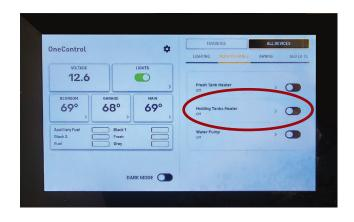
Circled in red, you will see the portion of the screen displaying the monitoring section for the tanks. The OCTP is hard wired into the RV and is powered by the 12-volt system. If the OCTP goes into sleep mode, you can wake it by pressing the button located just to the bottom of the panel. Please See <u>Section 16</u> for more detail on OneControl.
