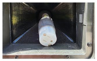
To operate, open the locked accessory door and carefully pull the extension out. To retract the extension, lightly pull to disengage the lock and allow the reel to retract.
