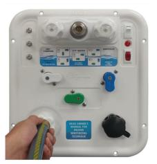
5. **TURN ON** the water pump and fill the fresh tank with the full amount of sanitizing solution. You can turn the water pump on at the Convenience Center (picture below left) or the OneControl Panel (picture below right):
