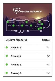
If yellow, RV Health Monitor has detected a variation in operating range that may benefit from close inspection or service. It may also mean a battery is severely depleted or is in poor health.
