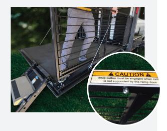
10. Pivot the door side rail towards the RV until it meets the other rail. Once the off door (driver) side rail is close to the other, you will need to slightly lift the rail to set it into its proper closed position.
