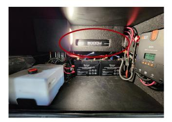
The purpose of this inverter is to invert 12-volt DC auxiliary battery power to usable 120-volt AC power for the RV. Power is inverted within two stages. Within the first stage, 12-volt DC power is amplified and converted to 300-volts DC. Within the second stage, the high voltage is converted into the needed watts (power) required to invert to 120-volts by using a form of transistor technology.
