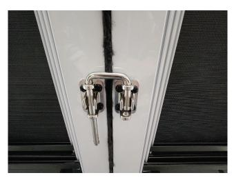
This lock provides some security and also acts as a securement for the door assembly when transporting the RV.
