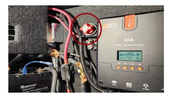
When auxiliary power is not needed for short term, the travel battery disconnect should be utilized.
