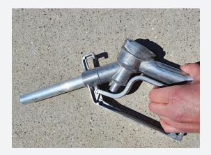
8. Once the tank is full, release the fuel handle, return the nozzle to the compartment, and turn OFF the fuel pump switch. Once you turn the pump off, you will hear the pump operate in reverse. This is to empty any remaining fuel found in the hose or dispensing nozzle.
