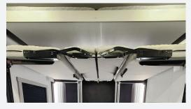
3. Press and hold the DOWN button until the limit switches stop the lift's movement. Your bunks will now be in the down position.
