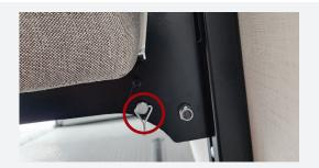
3. Pull up slightly on the bracket arm, then pull in an outward motion. This will release the sofa from the bracket and will allow the sofa to pivot downward.
