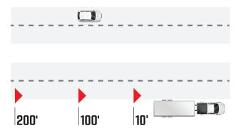
**1st indicator**: 10 feet (3.05 m) behind the RV driver's side also referred to as off door side.
