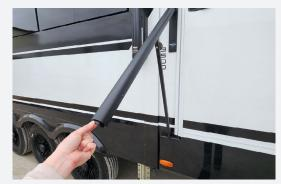
2. There is an inner and outer channel that comprises the handrail. Once the handrail is extended in step (1), firmly grab the inner channel located at the bottom of the handrail and pull it down and outward until the inner channel is fully extended. When complete, your handrail should look like the photo below.
