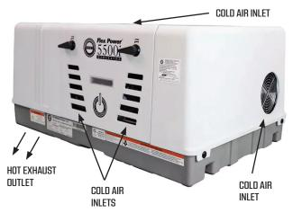
However, the cool air intake and hot air discharge have potential to recirculate hot air. Lack of intended paths for airflow, positioning of the generator, compartment spacing around the generator, and long skirting can cause hot exhaust to be ingested into the intake of the generator, an effect known as "hot air recirculation."
