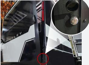
2. With one hand on the ramp door, insert the key and rotate counter-clockwise to release,
