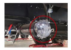
The picture below shows the sewer hose storage tube. The tube is capable of storing two sections of hose. The valve ends of the hose have to be removed prior to storage.
