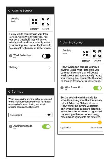
After turning Wind Sensors on in the App, they appear in the OCTP. Access them through the arrow in the upper right of the Awning's controls in the Motion page.
