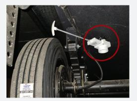
4. **ENSURE** the low point drains are closed. See picture, top right.
