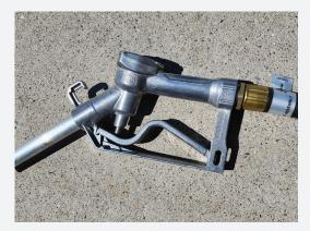
7. Begin filling by squeezing the trigger on the fuel nozzle. Be careful not to overfill the vehicle's or equipment's fuel tank. If spillage occurs, clean the area immediately.
