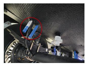
The purpose of these lines is to alleviate pressure as it is built within the tank, or to prevent the tank from overfilling when being filled. On occasion, you may see water being expelled from these lines if the tank is overfilled, the RV is parked on an incline, or when from stopping and starting while traveling. This is normal and should not pose a concern.
