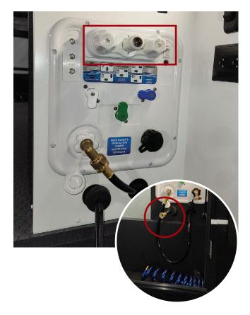
The second spray port is located on the wall of the pass-through storage on the door (passenger) side of the RV. The below photo shows the spray port and its location.
