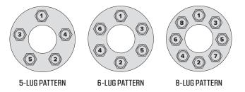
Determine the correct torque and torque sequence for each stage and use the Final Torque Specification Table shown below.
