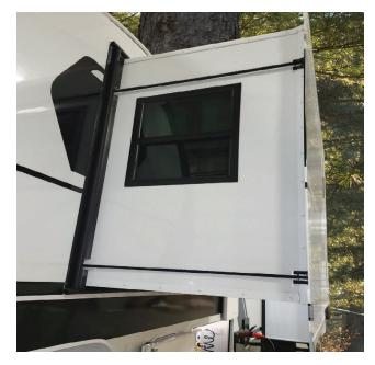
As you can see in the picture directly above, the SlimRack system has two gear racks on either side of the slide room.
