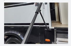
3. Reverse steps (2) and (1) above to stow the handrail for travel. Be sure to fully seat the handrail so that the magnet engages to the side wall of the RV and insert the travel pin.
