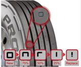
THE WEAR SQUARE™ (VISUAL WEAR INDICATOR) ALLOWS YOU TO QUICKLY SEE THE APPROXIMATE TREAD LIFE REMAINING ON YOUR TIRES AND CAN ASSIST IN DETECTING WHEEL ALIGNMENT ISSUES WITH YOUR VEHICLE.
