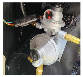
After the LP cylinder is refilled, remember to reconnect the pigtail line and secure the LP cylinder with the provided straps. If you would like notice before the regulator begins to pull from this cylinder, leave the valve closed. This will prevent the regulator from switching to the opposing LP cylinder without notice.
