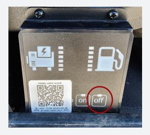
9. After 2 minutes of inactivity, the fuel station control panel will return to the locked mode.
