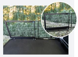
9. The off door side rail also contains the rail kit portion for the front or top of the ramp door. Pivot the front rail into place and engage the latch as indicated in the below photo.
