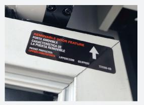
2. Just above this label, you will find a silver plate on the door bracket with two screws. Using a phillips bit, remove the two screws, fully exposing the opening on the upper bracket
