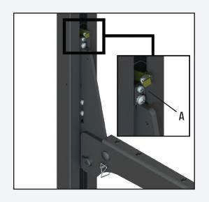
3. Run the lift system until both bunks are in the closed or up/stowed position.
