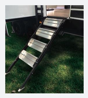
4. Grab the top of one of the step treads and pull towards you until the steps are fully seated in the down position. The steps should look like as shown in the picture below.
