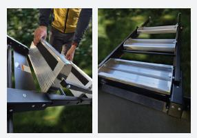
b. Press the two push releases in, and lift the stair up.
