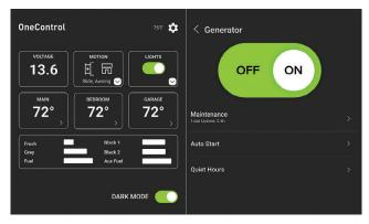
If you set the generator to start automatically, consider setting quiet hours. This will prevent the generator from turning on during a campground's observed quiet time.
