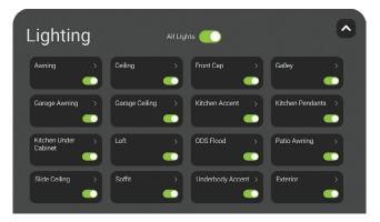
To turn lights ON or OFF, press the switch in the lower right corner. To access premium controls, press anywhere else on the button. Premium controls include dimming, color, sleep timer and behavior like pulsing and frequency. If your RV has more than 16 lights, you may swipe to the left to access them.
