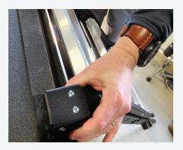
c. Before storing, the legs on the stairs will need to be fully retracted. This can be performed by removing the leg pins and sliding the legs to the last hole available and then reinserting the pin.
