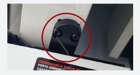
4. Once aligned, carefully tilt the panel back towards the RV. As the panel is released from the upper bracket, the full weight of the panel set will be in your hands. If assistance is needed, be sure to ask for assistance before releasing the panel from the bracket.
