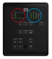
The red circled portion of the monitor panel shown above indicates the holding tank level information. In addition, it also will display voltage of the auxiliary battery. The battery charge information is shown on the portion of the panel circled in blue.
