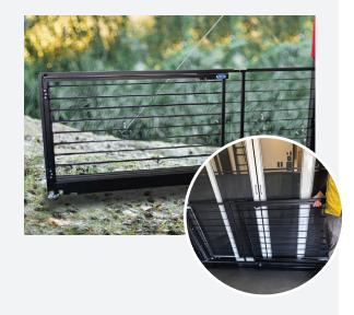
9. Locate the next foot latch on the door (passenger) side rail and press the latch down to release while pulling the rail straight back towards the RV until you hear the detention pin engage.
