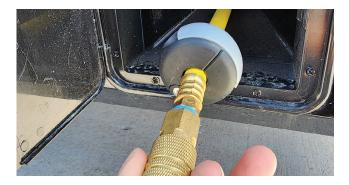
To operate, open the locked accessory door and carefully pull the hose out. To retract the hose, lightly pull to disengage the lock and allow the reel to retract.
