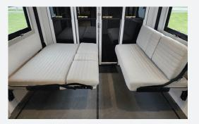
2. Remove the lockpins securing both bracket arms. These are located on the backside of the sofa. There will be one at each end of the sofa. Be prepared for the weight to shift as you remove the second pin from the sofa bracket.
