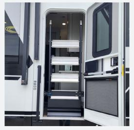
2. While holding on to the step, pull the blue lever to release the step from the door jamb. See the picture below displaying the blue handled latch.
