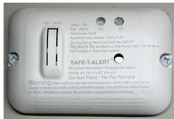
THE CO AND PROPANE GAS ALARM. SEE SECTION 4G FOR ITS LOCATION IN THE RV
