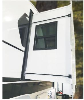
SlimRack system has two gear racks on either side of the slide room.
