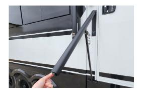
There is an inner and outer channel that comprises the handrail. Once the handrail is extended in step (1), firmly grab the inner channel located at the bottom of the handrail and pull it down and outward until the inner channel is fully extended. When complete, your handrail should look like the photo below.
