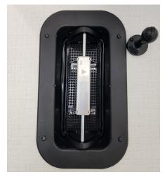
Locate the fuel switch found at the fuel station control panel. If the panel is in Sleep/Locked mode, press either the ON or OFF button. To unlock the panel press and hold the OFF button until the ON feature begins to blink.
