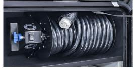
To release the shore cord, use the switch and guide the cord out until the full length of cord is freed from the reel.
