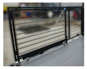
The off door side rail also contains the rail kit portion for the front or top of the ramp door.
