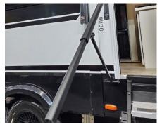
3. Reverse steps (2) and (1) above to stow the handrail for travel. Be sure to fully seat the handrail so that the magnet engages to the side wall of the RV and insert the travel pin.
