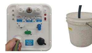
4. Push "**PUMP**" switch to turn on pump.
