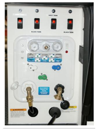
The second spray port is located on the wall of the pass-through storage on the door (passenger) side of the RV. The below photo shows the spray port and its location.
