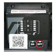
9. After 2 minutes of inactivity, the fuel station control panel will return to the locked mode.
