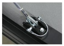
3. After locating these plates, remove the D-ring pin holding the cable in place.
