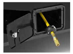
To operate, open the locked accessory door and carefully pull the hose out. To retract the hose, lightly pull to disengage the lock and allow the reel to retract.
