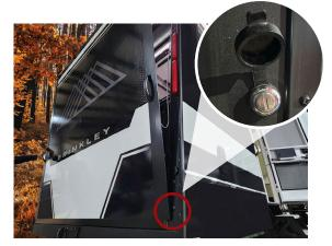
2. With one hand on the ramp door, insert the key and rotate counter-clockwise to release, or unlock, the ramp door.
