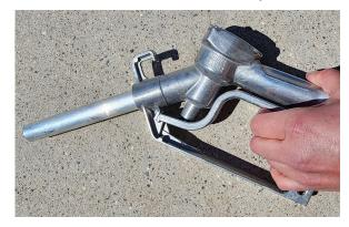
8. Once the tank is full, release the fuel handle, return the nozzle to the compartment, and turn OFF the fuel pump switch. Once you turn the pump off, you will hear the pump operate in reverse. This is to empty any remaining fuel found in the hose or dispensing nozzle.
