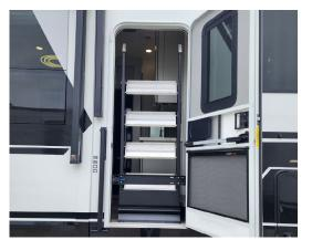
2. While holding on to the step, pull the blue lever to release the step from the door jamb. See the picture below displaying the blue handled latch.
