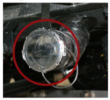
The picture below shows the sewer hose storage tube. The tube is capable of storing two sections of hose. The valve ends of the hose have to be removed prior to storage.
