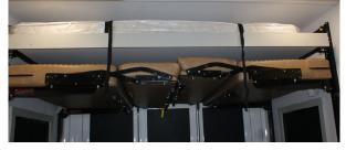
3. Press and hold the DOWN button until the limit switches stop the lift's movement. Your bunks will now be in the down position.
