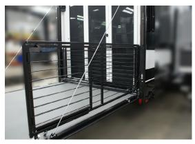
5. As the rail meets the edge of the ramp door, you will need extend the telescoping portion of the rail kit to the outermost corner of the ramp door. This is performed by pushing in the detent pin in the top rail (see A below for location) and then grabbing the rail and guiding it towards the direction of the stairs.
