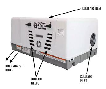
However, the cool air intake and hot air discharge have potential to recirculate hot air. Lack of intended paths for airflow, positioning of the generator, compartment spacing around the generator, and long skirting can cause hot exhaust to be ingested into the intake of the generator, an effect known as "hot air recirculation."
