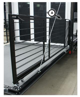
6. Once the rail is fully extended, engage the latching mechanism at the end of the railing as shown in the picture below.
