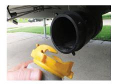
2. Open black waste holding tank and leave open to allow black tank to drain.
