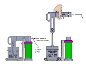
• Reverse steps 1 and 2 to reassemble your RV once the valve is back into its closed position and the pin is reinserted.
