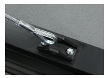
Place the cable eyelet between the plate verticals and insert the provided D-ring in the correct orientation and ensure it is secured with the supplied cotter pin. Please see below.
