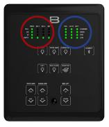
The red circled portion of the monitor panel shown on the previous page indicates the holding tank level information. In addition, it also will display voltage of the auxiliary battery. The battery charge information is shown on the portion of the panel circled in blue.
