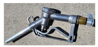
7. Begin filling by squeezing the trigger on the fuel nozzle. Be careful not to overfill the vehicle's or equipment's fuel tank. If spillage occurs, clean the area immediately.
