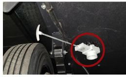
4. ENSURE the low point drains are closed. See picture, top right.
