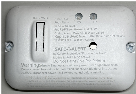
THE CO AND PROPANE GAS ALARM.
