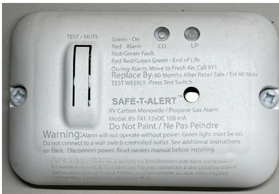
THE CO AND PROPANE GAS ALARM.
